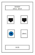
NOTE: When installing a coax port on a recessed (Semtron) faceplate with 3 jacks, use a 4-position plate with a blank. Do NOT install coax on the bottom of a 3-position recessed plate.
