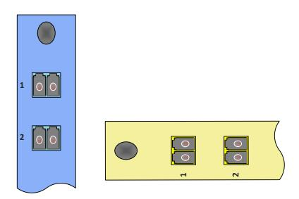
For vertical pack, fiber strand 1 is in the upper left. For horizontal pack, fiber strand 1 is in the lower.
