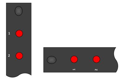
For vertical pack, fiber strand 1 is on top. For horizontal pack, fiber strand 1 is on the left.
